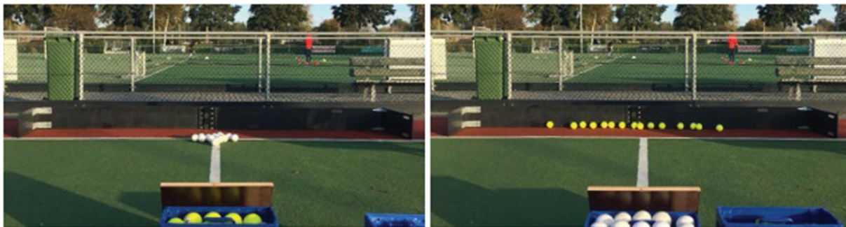
Figure 1. End position of the ball. Left picture: regular ball; right picture: modified ball. The regular ball rolled straight resulting in small dispersion of the end point, while the modified ball path was less predictable resulting in large dispersion of the end point.
